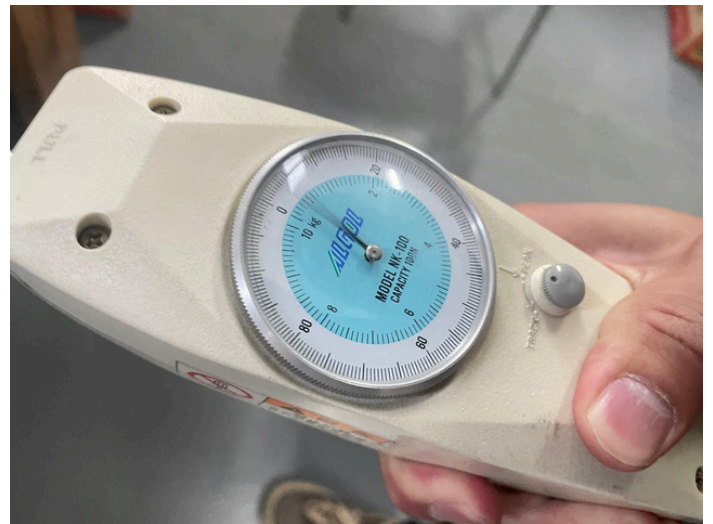
Pull test on power cord
