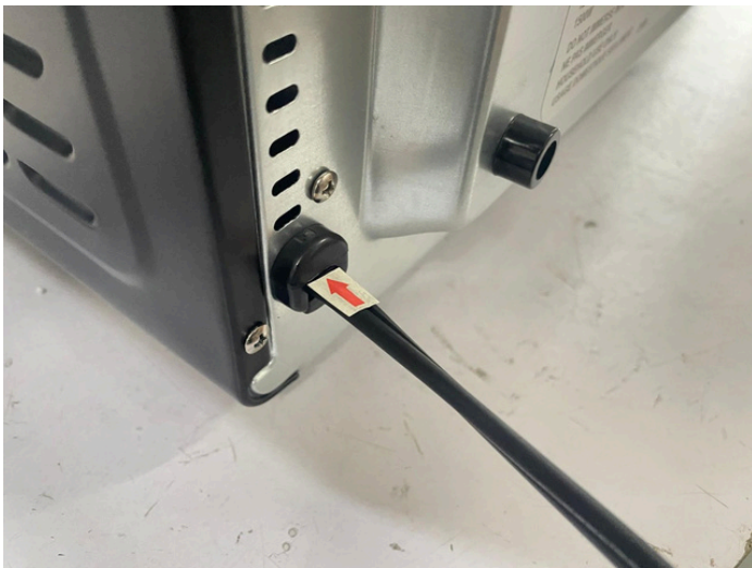
Pull test on power cord
